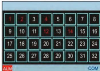
A 32-position grid where each numbered position is related to its equivalent alarm or event. When an alarm is active, its number will be displayed in red on this screen.
